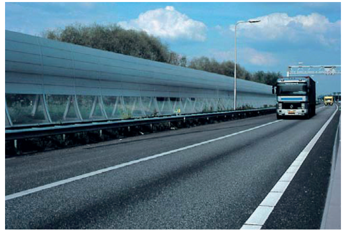
Lärmschutzwand, Terbregseplein PLEXIGLAS® Soundstop GS Reynolds Special Products B. V. Lelystad
